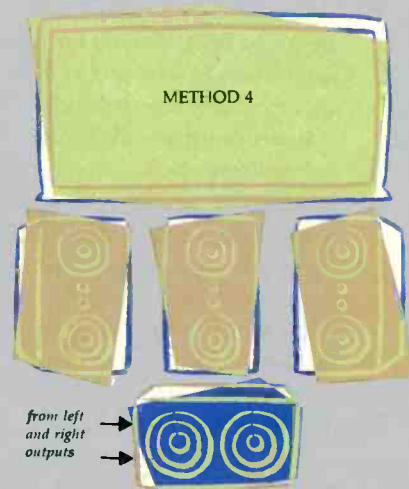
Fig. B4—Left, right, and center speakers used with subwoofer fed from undecoded left and right stereo signals.
