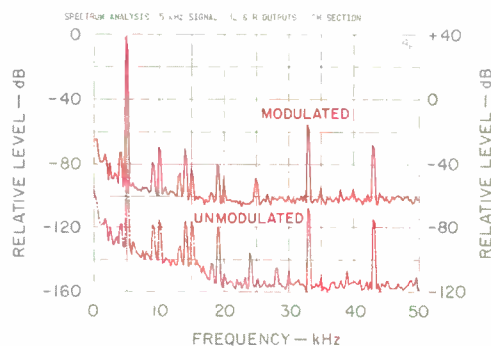
Fig. 6—Spectrum analysis, showing FM stereo crosstalk and distortion products. Use right-hand scale for bottom curve.
