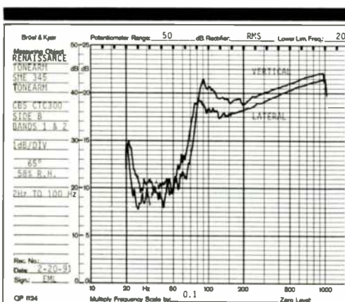
Fig. 4—Response to vertical and lateral modulation from 2 to 100 Hz (slow sweep).
