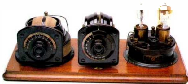
Atwater Kent Model 3925 (1922) AK's first factory-wired receiver in the "breadboard" style, selling for $52. (Prior sets were sold as components and wired by the buyer.) The two-tube unit, with an r.f. amp and a detector/audio amp, required a battery as well as headphones. The buyer added a vario-coupler to make it a regenerative circuit, thus saving AK from infringing on the Armstrong-RCA patent. COURTESY OF RALPH AND ELINOR WILLIAMS.
