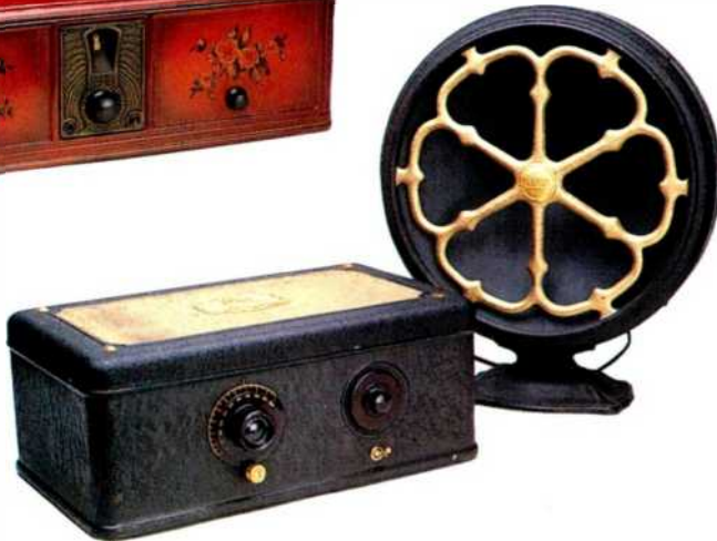
Atwater Kent Model 40 with Speaker Model E (1928) A seven-tube TRF receiver, made during AK's most productive period. This metal-cased unit sold for $77 (without tubes). COURTESY OF ATWATER KENT FOUNDATION.
