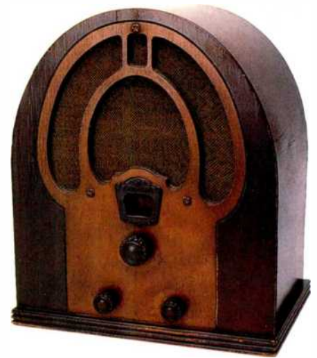
Philco Model 81 (1933) A four-tube superbheterodyne receiver. Designed for low cost because of the Depression, it sold for about $25. Seventy percent of the radios sold in 1935 were of this "cathedral" style. COURTESY OF BILL AND CAROL DIGEL.
