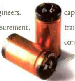
Filtering capacitors for the power supply are copper shielded, preventing mutual interference.
