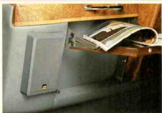
The most visible signs of stereo are the mini-plates behind the front seat.
