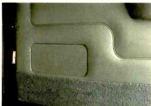
The openings for the speakers in the front doors were originally for storage compartments.
