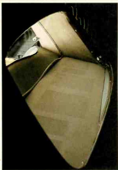
Covered with cloth that matches the car's interior, the rear-deck speakers and the subwoofer vents are almost invisible.
