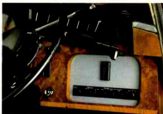
The chauffeur operates the system with a Nakamichi preamp and the Concord CD changer's remote control and display.
