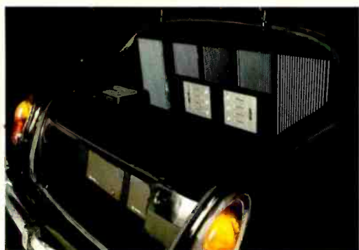
A trunk full of goodies, with amps, crossovers, a hidden CD changer, and the videocassette player above, power supplies for stationary use below.
