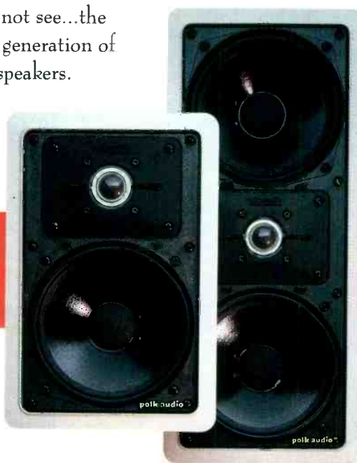
The AB 700 requires a 9 3/4" H x 6 1/4" W x 3" D cutout. The AB 800, with two midbass drivers, requires a 15 1/2" H x 6 1/4" W x 3" D cutout.
