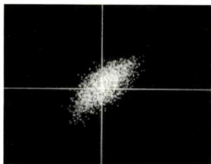
Fig. 7—Interchannel phase difference, using pink noise from B & K 2011, band 7.
