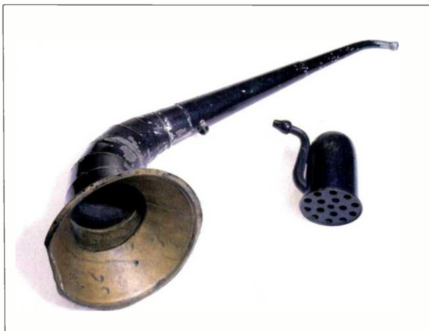
Ungainly acoustic horns, in a variety of shapes and sizes, provided 10 to 20 dB of gain — and required no batteries.
