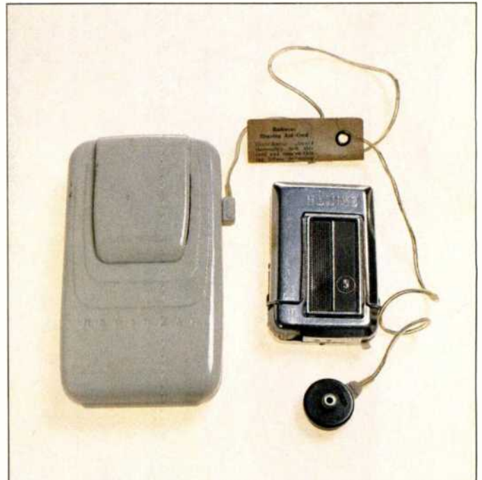
The tube-amplified aids of the 1940s (left) quickly gave way in the '50s to more compact, transistorized models (right).
