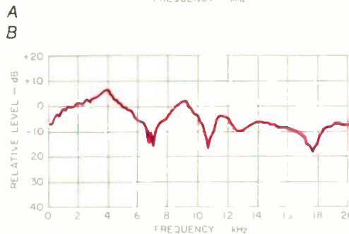
Fig. 3— Pinna response for sound source at 90° azimuth and 15° above ear level (A) and at 180° azimuth (directly behind the head) and below ear level (B). Note the high-frequency attenuation in (B). (After Rodgers.)
