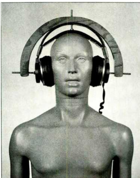
Fig 11— The KEMAR mannequin, with a zero-static-force restraining yoke holding headphones under test. (From Russotti, Santoro, and Haskell.)
