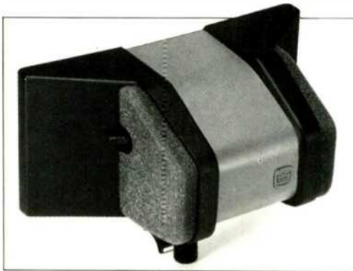
Fig. 16— Crown International's SASS quasi-binaural mike configuration, using PZM microphones.
