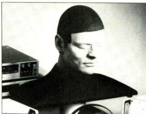
Fig. 15— The Aachen dummy head, which is compatible with loudspeakers, and its associated hardware.
