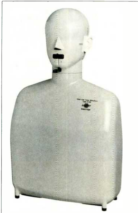
Fig 10— B & K's Type 4128 head and torso simulator.
