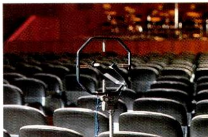
Symmetrical 6-Point Sound Field Measurement Microphone Set
