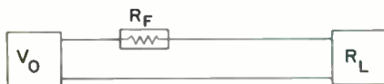
Fig. 4—Circuit for the series fuse often used for speaker protection. Possible worst-case distortion figures for this circuit are given in Table VI.
