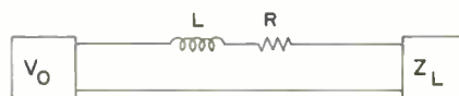
Fig. 2—Simplified circuit for a "good" amplifier driving a cable and loudspeaker load. Critical frequencies for this circuit are summarized in Table V.
