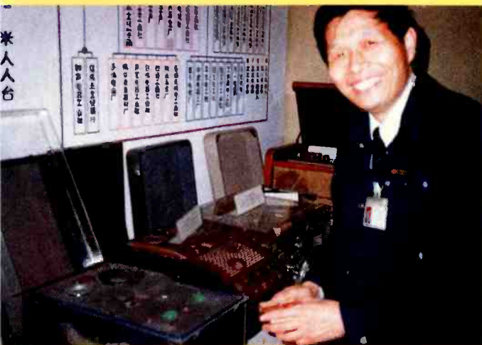
Yang He Ming, director of the Shanghai Tape Recording Equipment Factory, poses with China's first wire recorder, made by the factory in 1951 (far left). Next to it are three open-reel machines produced by the factory from 1953 to 1973. The second and third machines from the left were designed to use paper-based tape.
