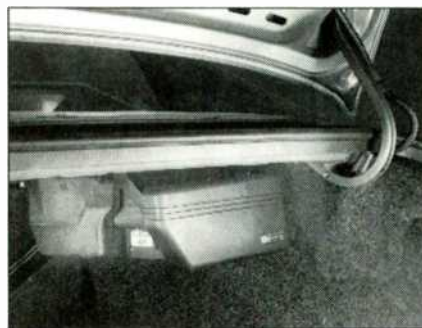
New subwoofer enclosure provides deep bass without taking up much trunk space or interfering with the fold-down seat.
