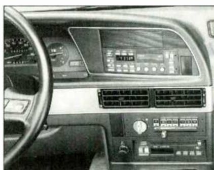
Head unit is mounted high in the Thunderbird dash for easy access, but the optional CD player mounts about a foot below.
