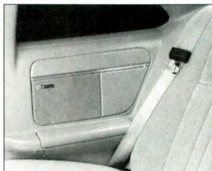
In the Thunderbird and Cougar, rear-speaker placement gives back-seat passengers about the same sound quality as front passengers get.
