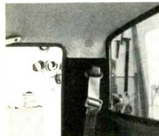
(Left) 741 system in rear of pickup cab includes 4" woofer and Varmount tweeter, the latter concealed under headliner. (Right)
