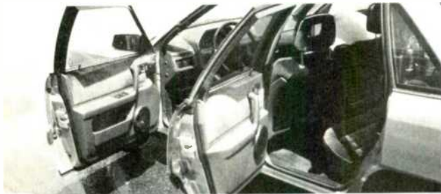
This unusual installation features three-way 763 component systems in front, with 6 1/2" subwoofers installed in doors, Varmount® tweeters surface-mounted on doors, and 4" midranges in dash. 767 6 1/2" two-way uniaxial systems in rear doors.
