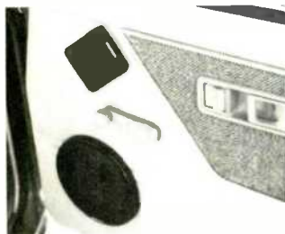
Boston 761 two-way component system in each door includes a 6 1/2" woofer and angled Varmount tweeter.
