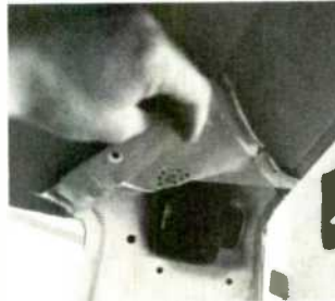
(Left) 741 system in rear of pickup cab includes 4" woofer and Varmount tweeter, the latter concealed under headliner. (Right)
