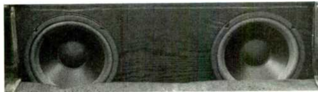
Boston 761 two-way component system in each door includes a 6 1/2" woofer and angled Varmount tweeter.
