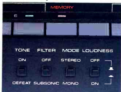
Subsonic filters utilize power efficiently, eliminate distortion, protecting speakers from subsonic frequency damage.
