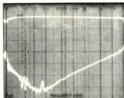
Fig. 3—FM frequency response (top trace) and separation vs. frequency.
