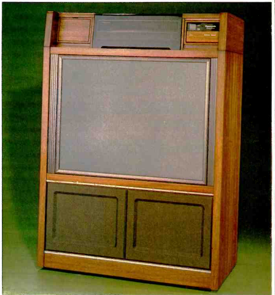
Panasonic's 40-inch, rear-projection TV uses a three-tube, three-lens system.
