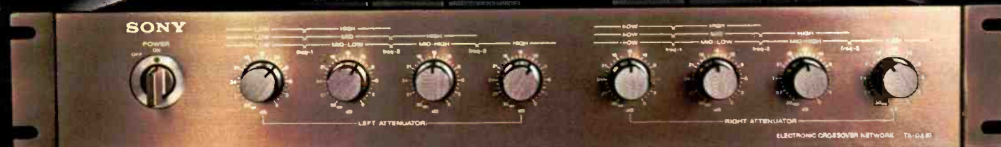
TA-D88B ELECTRONIC CROSSOVER NETWORK: Plug-in filter modules offer choice of 12 crossover points / Bessel-function filters provide up to 24 dB per octave slopes / Up to -30 dB attenuation range / 'Dual mono' configuration, with subchassis isolated power supply.
