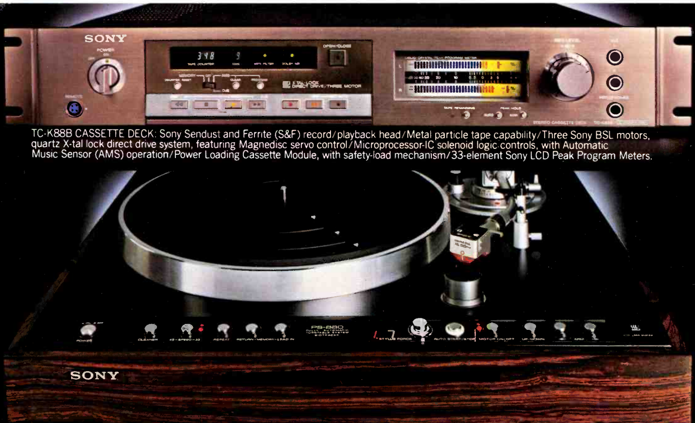
PS-B80 TURNTABLE: Velocity Feedback (VFB) electronically controlled tone arm system allows automatic tracking, antiskating, and tone arm damping operation/Microprocessor-programmable functions and replay flexibility/Quartz X-tal locked, fully automatic DD turntable, with high-torque BSL motor and Magnedisc servo control/SBMC chassis material, with height-adjustable viscous feet.
