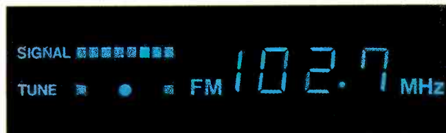
2. Behind this digital readout is a quartz-locked tuning system. More accurate, but it still requires a center channel tuning meter. And it still requires manual tuning.
