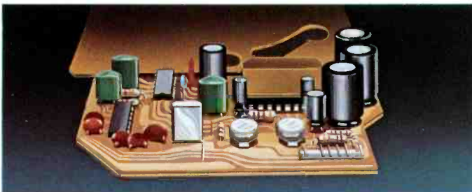
THE PIONEER QUARTZ PHASE LOCK LOOP SYSTEM. BY AUTOMATIC MONITORING, ROTATIONAL SPEED IS KEPT CONSTANT TO REDUCE WOW AND FLUTTER.
