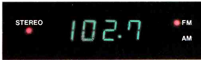
1. Behind this digital readout is a conventional tuning system. It requires a center channel tuning meter and manual tuning.
