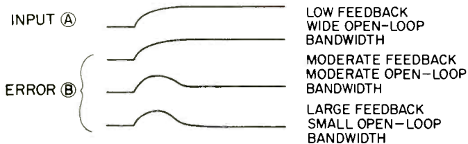
Fig. 6—A model of the feedback amplifier showing the error time response to a bandlimited step input for various combinations of feedback factor and open-loop bandwidth. Closed-loop bandwidth is held constant, and feedback is varied by changing only A2. Input level is assumed to be zero prior to the step.
