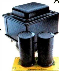
DC power supply found on the most expensive receivers.
