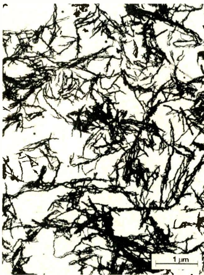
Fig. 3 — Particles used in TDK metal-particle tape.
