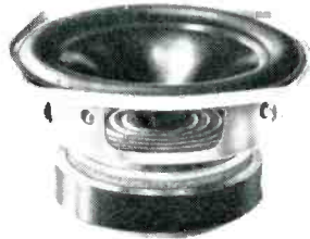
KEF B110 SP1003 A 5 inch drive unit, using the same diaphragm construction as the B200 with visco-elastic damping layers to ensure low colouration. Frequency range 55 to 3500Hz.
