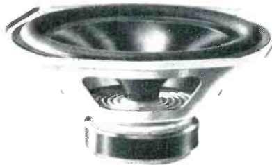
KEF B200 SP1014 An 8 inch low frequency driver with a diaphragm of rubber modified polystyrene. Frequency range 25 to 3500Hz.
