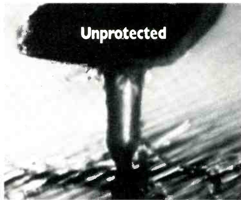
Magnification shows the record vinyl wearing away.
