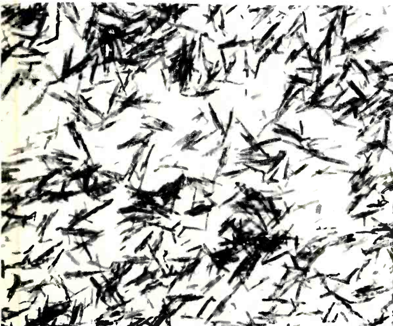
Fig. 1—An electron photomicrograph of a typical iron oxide magnetic material was made with a magnification of 45,000. The average length of these particles is about 0.4 microns, and the ratio of length to width is six to one.
