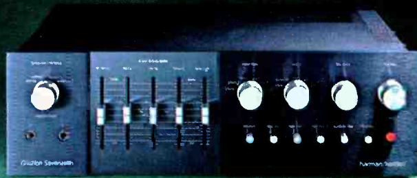
Citation 17 Preamplifier. Frequency response from below 3Hz to beyond 270,000Hz, -3dB. Less than 0.001% THD, phono preamp less than 0.002% THD.
