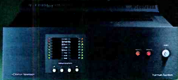
Citation 19 Power Amplifier. 100W min. RMS per channel into 8 ohms from 20Hz to 20kHz, with less than 0.08% THD. Frequency response from below 5Hz to beyond 140kHz, -3dB.
