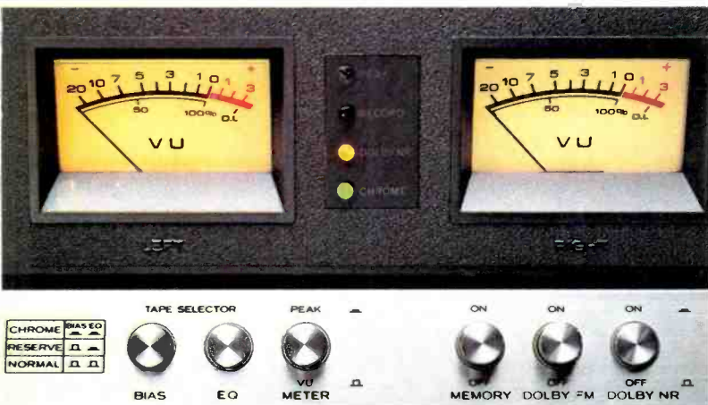
Switchable VU and Peak meters for better recordings.
