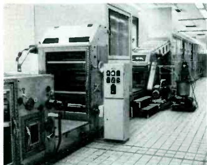
Coating plant —the dispersion is spread evenly and precisely onto a wafer-thin plastics carrier film.
