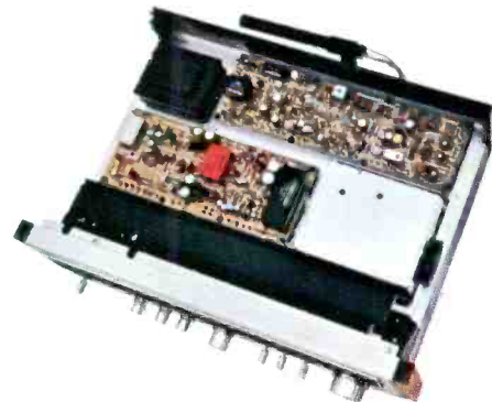
TX-9100 interior view. Chrome plated shielded front end housing and multiplex section.
