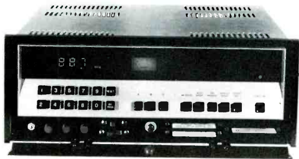
Fig. 1—Front of AJ-1510 with trap door panel opened.
