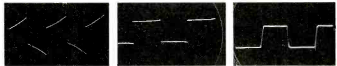
Fig. 9—Square-wave performance at A, 60; B, 1000, and C, 10,000 Hz.
