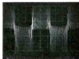
Fig. 6a—vert, 200 mV/div. Fig. 6b—vert, 5 mV/div. (54 dB separation)
