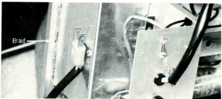
Fig. 2—The effective r.f. shielding.
