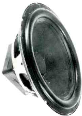
Fig. 4—Showing bass speaker used in the EPI-100. Note the large double magnet.
