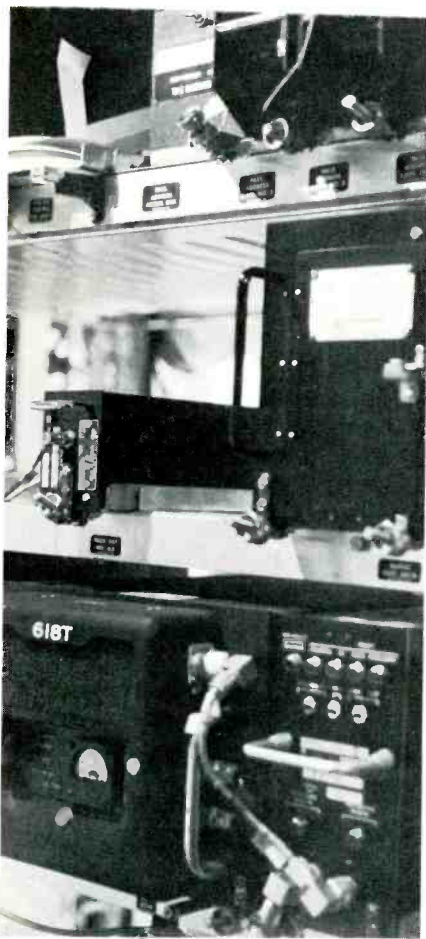
Fig. 8—Amid a whole array of electronic equipment under the floor are the main multiplexer (left center) and the tape reproducer (right center). Below it is the main PA amplifier which feeds the 61 Jenson speakers.
