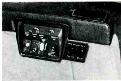
Fig. 6—Passenger's control unit, located in the seat armrest. Program selection, volume, reading light, and hostess call button are provided here, as well as control for reclining seat back and the new "lumbar" inflatable cushion for support to the passenger's lower back area.
