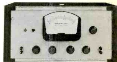
Amplifier Corp. of America Model 590-A—Lowest readable flutter: 0.01%. Test frequency: 3 kHz. $495.00.
