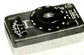
H. H. Scott Model 450 Sound Meter—Palm-sized sound level meter. Fully transistorized. Designed for ASA Standard S1.4-1961, A, B and C weightings. Range: 40 to 142 dB. Frequency range: 35 to 8000 Hz. Built-in crystal microphone. A.C. line calibration. $182.00.
