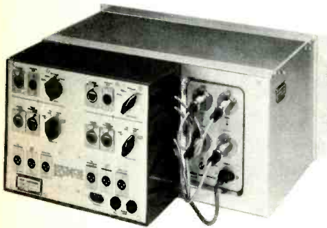
Fig. 3—Changeover system. Added to the back of Model A301, the changeover facility enables one unit to be used for recording and non-simultaneous playback on two tracks. Both remote control and manual control are provided.
