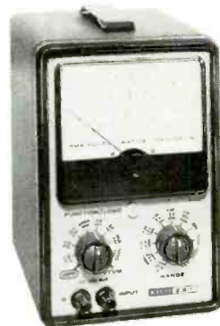
EICO Model 262 AC Volt/Watt meter—Voltage ranges: 10 mV to 1000 V rms; power range: 0.15 mW to 150 W. Incorporates tapped power resistor loads (4, 8, 16 and 600 ohms). $59.95 (kit); $89.95 (assembled).
