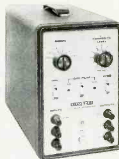
EICO Model 342—Generator provides both composite audio and FM r.f. outputs. External SCA. Separation: 30 dB min., 50 to 15 kHz. Crystal-controlled 19 kHz pilot. $175.00 (wired only).
