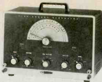
Heathkit Model IG-82 — Sine/square wave. 20 Hz to 1 MHz. Under 0.15 \mu s rise time. $53.95 (kit). Assembled Model IGW-47, $94.00.
