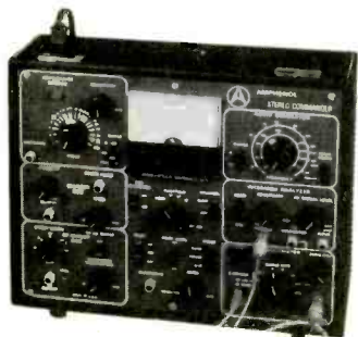
Amphenol Model 880 — Combination Tester—Seven test instruments are combined here: sine- and square-wave generator, FM multiplex generator, r.f. sweep generator, with 10.7 MHz marker, IM distortion analyzer (SMPTE standard), a.c. VTVM, and an impedance bridge. $329.95.
