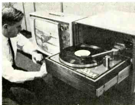
Fig. 1—The "Phonovid" still-picture/sound system is shown at left, playing a special LP record on a Garrard automatic turntable. At right is Sony's magnetic-type video disc, which records and plays back still pictures in black-and-white and color, as well as sound.
