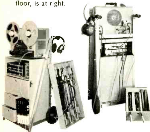
Fig. 2—Front view of the dolly with drawers partially open is shown at left. A rear view, with a microphone drawer on the floor, is at right.
