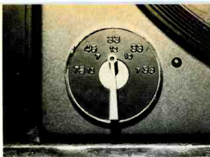
Fig. 4—Combined speed and record-size selector. (The SL-95 has 33 \frac{1}{3} rpm, 45 rpm and 78 rpm speeds.)
