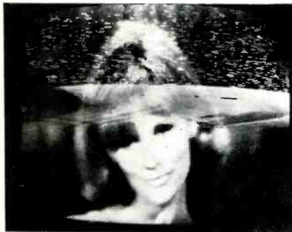
Fig. 1—Video tape recorded and played back at half speed ( 3\frac{3}{4} ips) as it goes over splice between iron oxide tape (top) and "Crolyn" tape (bottom).
