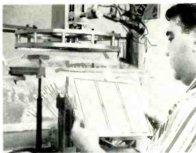
Fig. 2—Custom-built machine stretches and mounts diaphragm material to molded frame.
