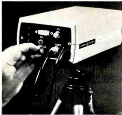
Fig. 3. The new General Electric type TE-23 CCTV camera is solid-state, and equipped with a crystal oscillator to provide optimum picture stability. Camera resolution is approximately 500 lines when displayed on a standard video monitor. Only two controls—an on/off switch and focus knob—provide simplicity and ease of operation.
