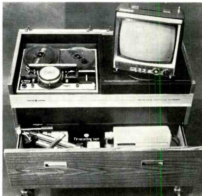
Fig. 1. General Electric's new video tape recorder mobile console encloses the system's three major components — a video tape recorder, a monitor and a closed-circuit TV camera, plus a complete set of accessories such as a tripod, microphone with lavalier and stand, ½ hour of recording tape and connecting cable.
