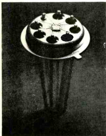
Fig. 1. Assembly of a typical integrated Circuit. Note that this model has eight connections. The \mu A703 has six external connections.
