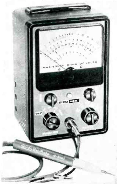
EICO 222 A general purpose ac-dc-ohms unit with a low-scale sensitivity of 3 volts full scale. A zero-center-scale feature is provided for null-type readings. A single multi-purpose probe is supplied for use with all measurements. Frequency response is 30 Hz to 3 mHz. Price is $27.95 as a kit and $42.95 wired.
