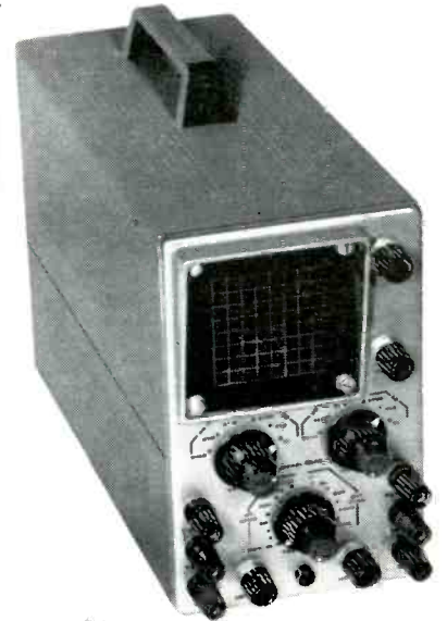
Heathkit 10-10 A 3" a.c.-d.c. scope specifically suited to audio measurements. Features identical vertical and horizontal amplifiers with a d.c. to 200 kHz response at the -2 dB point. Sweep is available from 5 Hz (lower with an external capacitor) to 50 kHz. Sensitivity is 0.1 V/inch, peak-to-peak. The phase shift between channels is less than 5 deg. Price is $89.95 as a kit only.
