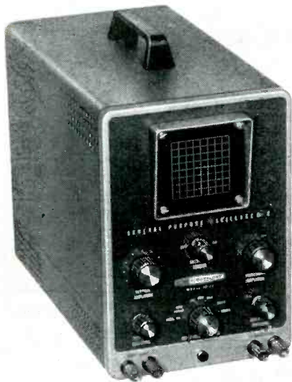
HEATHKIT 10-21 A general purpose compact scope. Has a 3" tube face. Features identical vertical and horizontal amplifiers with 2 Hz to 200 kHz \pm 2 dB response. Sweep generator range is 20 Hz to 100 kHz and sensitivity is 0.25 vol'ts/inch, rms. Price is $54.95 as a kit only.
