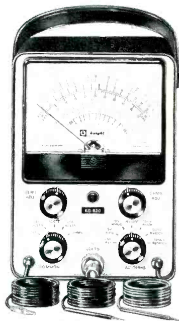
Knight KG-620 A general purpose ac-dc-ohms VTVM with a maximum full-scale range of 1.5 volts. Separate probes are provided for a.c. and ohms or d.c. volts. The meter may be set for center-scale measurements. Rms or peak-to-peak measurements may be made. Frequency response is 30 Hz to 5 mHz \pm 3dB. Price as a kit is $24.95; $39.95 is the wired price.
