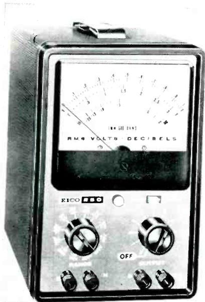
EICO 250 An a.c. VTVM designed particularly for audio measurement work. Maximum sensitivity is 1 mV full scale. Decibel range is -80 to +52 dB in 10-dB increments. Frequency response is \pm 0 dB from 10 Hz to 600 kHz. A switch converts the instrument to a high-gain amplifier with a maximum voltage output of 5 volts rms. Price is $49.95 as a kit and $79.95 wired. The same unit is available without the amplifier feature at $44.95 or $72.95. Also available is a reduced sensitivity VTVM that is also calibrated as a wattmeter. Price is $49.95 as a kit and $79.95 wired.
