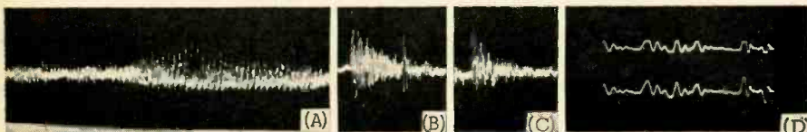
Fig. 1. Oscilloscope photos of various transients and effects of clipping: (A) Transient power peaks in musical passage; (B) and (C) examples of strong starting transients; (D) effect of clipping due to use of zener-diode limiter.
