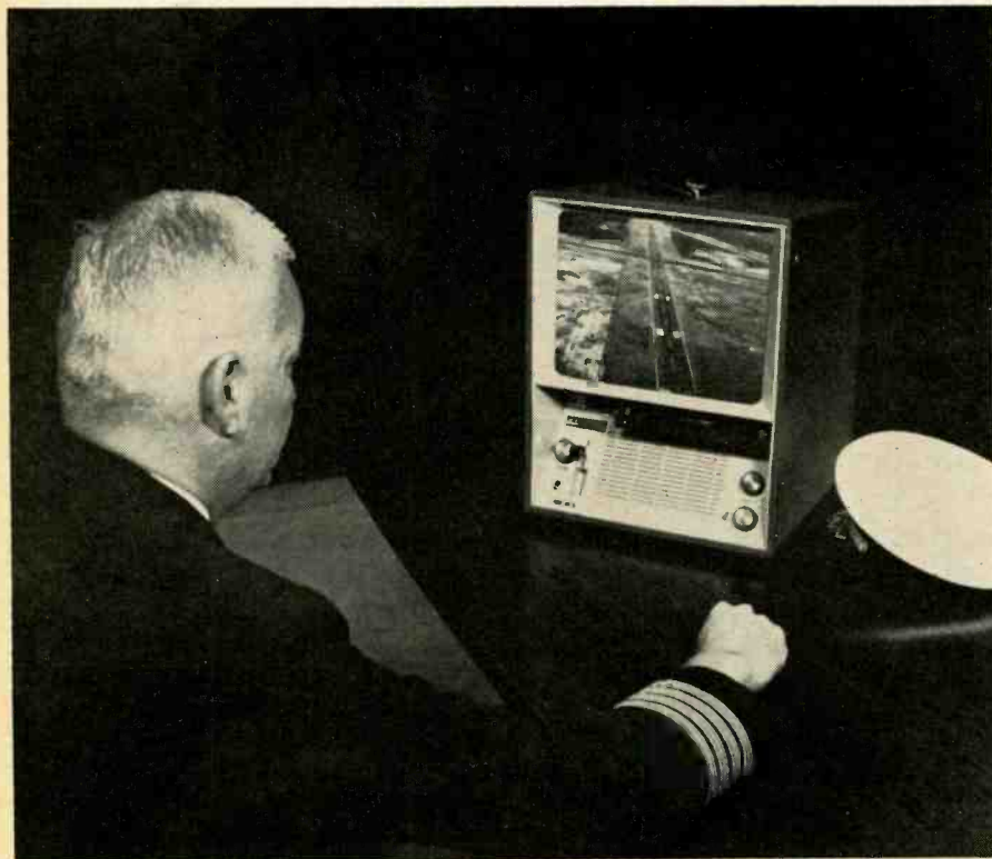
Packaged cartridge of 8-mm sound film provides airline pilot with a preview in color of his next airport destination.
