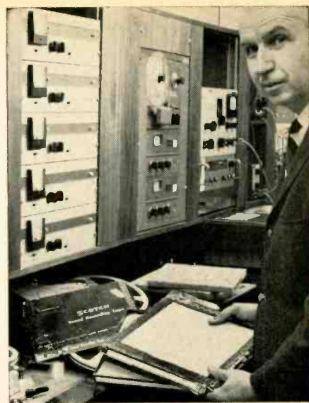
Fig. 1. Checking 1949 tapes of Bing Crosby and Al Jolson radio programs he recorded, Mullin finds no signs of aging. Tapes were stored in original, unsealed boxes for more than 15 years in garages in California heat and Minnesota cold. When played, sound reproduction was excellent. (Photo courtesy 3M.)
