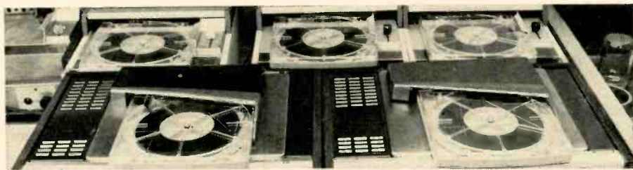
Fig. 2. Tape-punishing setup at 3M testing laboratory in St. Paul. Tapes are fashioned into continuous loops and are run 24 hours a day, giving wear equivalent to 100 years of normal use without appreciable change in performance of tapes. (Photo courtesy 3M.)
