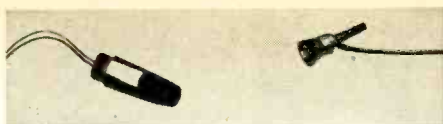
Fig. 6. Reed man Ted Nash's alto saxophone mouthpiece is "transduced" from tiny wires directly under reed. Horn mouthpiece wiring begins immediately under lip. Notches are made, then re-filled after wire is added.
