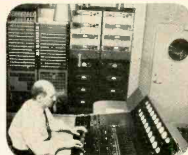
Banks of Altec 128B Amplifiers used for PLAYBACK monitoring by Universal Recording Corp., Chicago.
