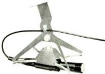
ALTEC 688A OMNIDIRECTIONAL DYNAMIC MICROPHONE —$90 net. Extremely uniform response from below 35 to over 20,000 cycles. Highly efficient. Low hum pickup. Shown in an Altec 181A Boom Mount. Output Impedance: 30/50, 150/250 and 20,000 ohms (selection by connections in microphone cable plug). Output Level: -55 dbm/10 dynes/cm 2 . Hum: -120 db (Ref.: 10 -3 Gauss). Dimensions: 1 1/8" diameter at top (1 1/2" largest diameter), 7 1/2" long not including plug. Weight: 8 ozs. (not including cable and plug).
