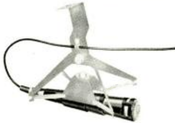
ALTEC 689A CARDIOID DYNAMIC MICROPHONE —$108 net. High front-to-back discrimination for an average of over 20 db from 40 to over 16,000 cycles. Virtually flat response throughout this frequency range. Output Impedance: 30/50, 150/250 and 20,000 ohms (selection by connections in microphone cable plug). Output Level: -54 dbm/10 dynes/cm 2 . Hum: -120 db (Ref.: 10 -3 Gauss). Dimensions: 1 1/2" diameter at top, 7 1/4" long not including plug. Weight: 11 ozs. (not including cable and plug).
