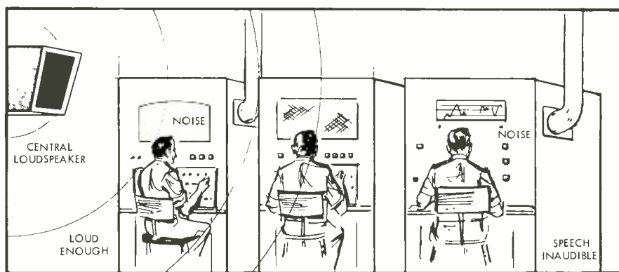
Fig. 5. A noisy space may be difficult to cover using a central loudspeaker system.
