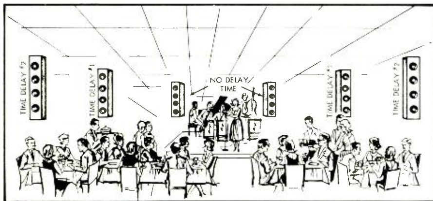
Fig. 4. A low-ceilinged night club space where a distributed line source system employing time delay may be applicable.
