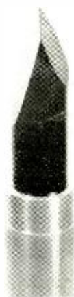
Fig. 1. CBS Laboratories MLS-915 stylus for recording 15-deg. angle with a Westrex 3C cutter.
