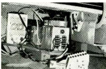
Fig. 10. Audio amplifier, multiplex adapter, and d.c.-d.c. converter in position under rear deck of car.
