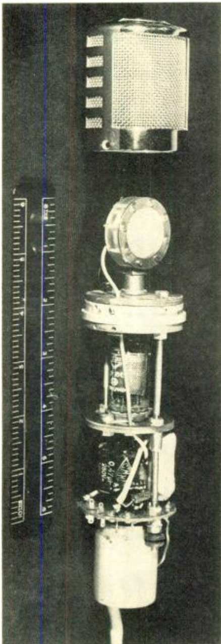
Fig. 9. Internal construction of one of the microphones. The plate-to-line transformer (balanced 30-50 ohms) is at the lower end. Note that the 2-in. diameter metal case and bottom cap are not shown.
