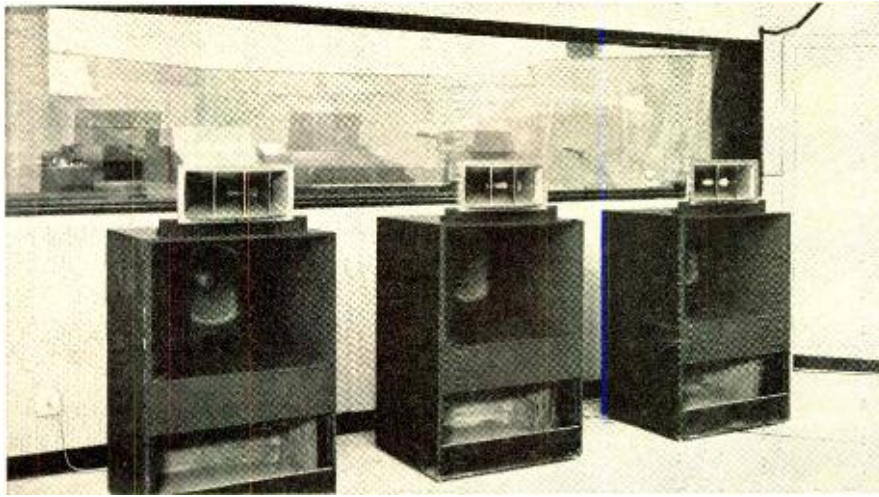
Studio view of three A-7 speaker systems used for 3-channel PLAYBACK monitoring at United Recording Studios, Hollywood, where many famous musical stars do their recording.
