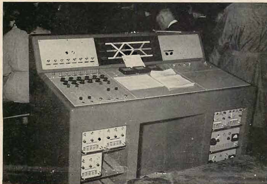
Control console used in the Grand Salon of the Palais d'Orsay Hotel for demonstrations. This unit is arranged for three channels, and the pattern at the top shows the channel routing at any given control settings.
