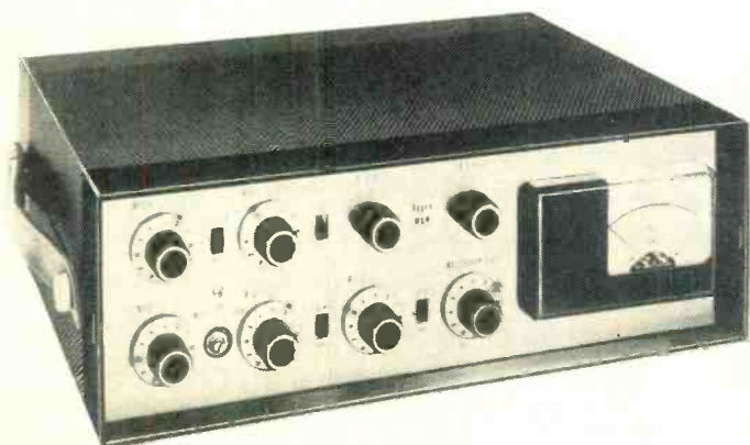
Fig. 3. Bogen MXM mixer-preamplifier. This type of equipment is ideal for stage use because it can feed any power amplifier and provides extremely flexible mixing as well as a meter for visual monitoring.
