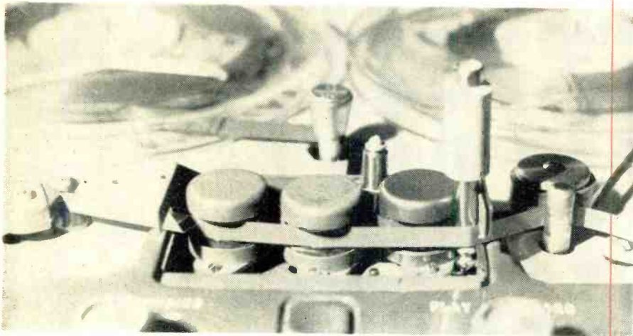
Fig. 2. Front view of tape threading technique.
