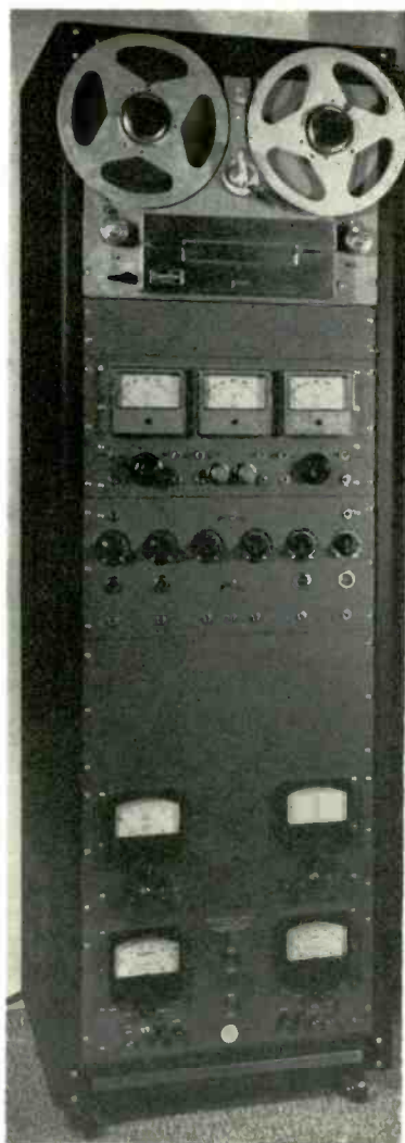
Fig. 5. Rack-mounted stereo record/playback system constructed by the author.
